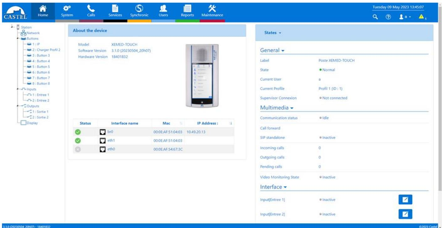
The screenshot shows the web interface of the XE2 MED TOUCH station. The top navigation bar includes Home, System, Calls, Services, Synchronic, Users, Reports, and Maintenance. The main content area is divided into three sections:
